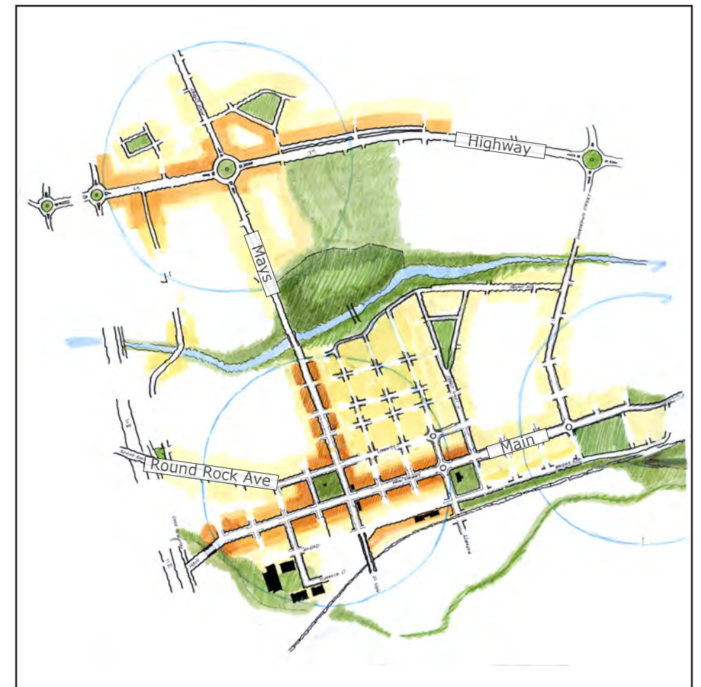
Initial Master Plan concept diagram sketch showing areas of intensity, critical streets, open space (in green), 1/4 mile walk circles, and civic buildings (in black).
